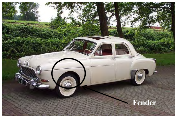
Figure 2.3: Renault Frigate one of example car using pontoon fender after the introduction from Earl and Cadillac (Heacock, 2014).
