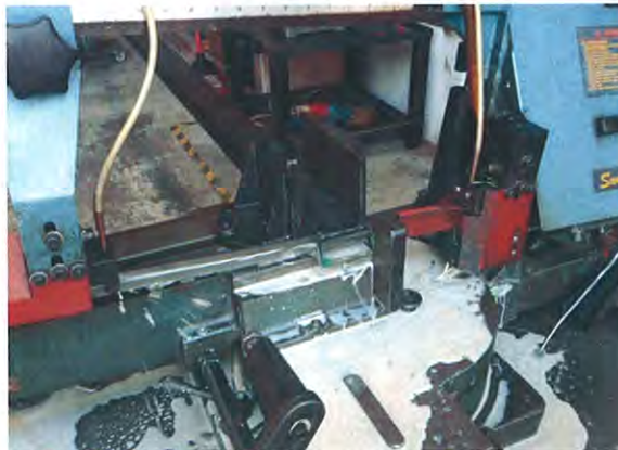
Figure 3.3: Cutting process using bend saw
