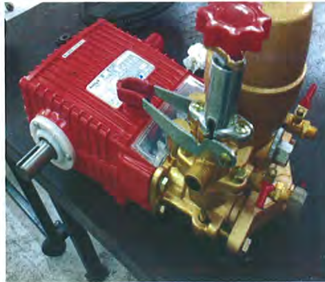
Figure 4.2: Wu Li-W-45B hydraulic pump
