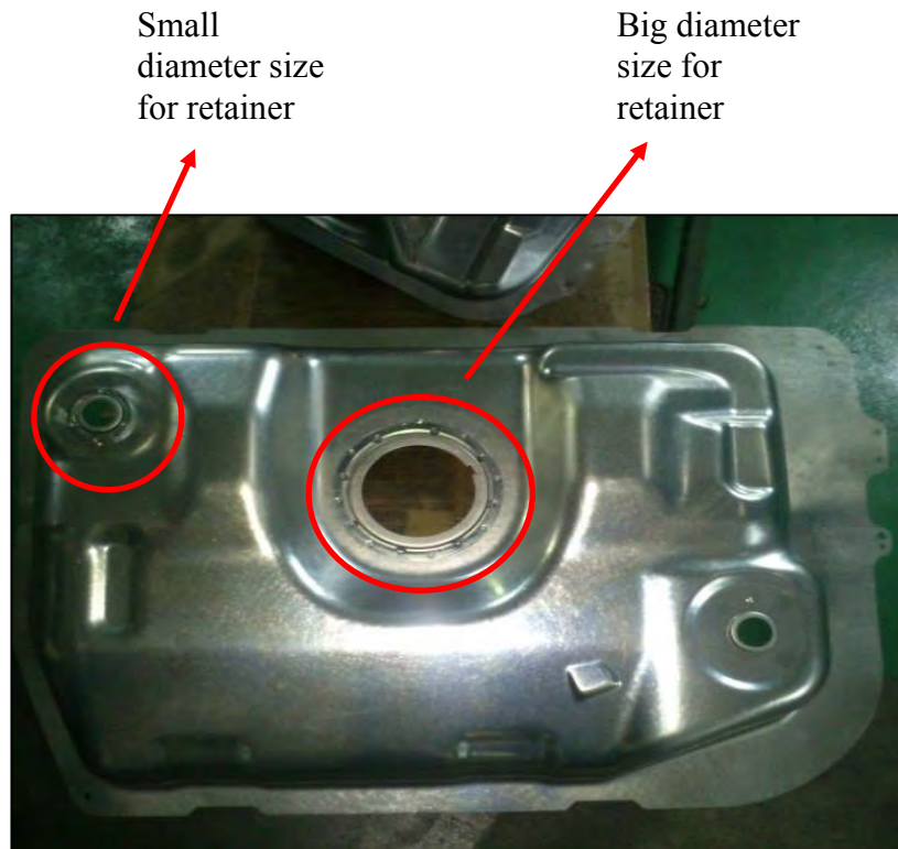
Figure 1.2: Fuel tank upper that assembled with automotive retainer. (Source : United Vehicles Industries Sdn. Bhd.)
