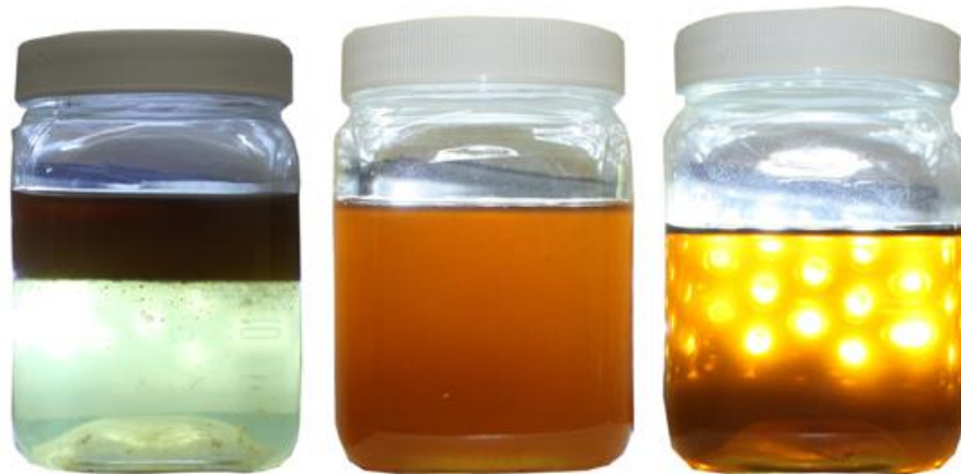
Figure 2.: Example water contamination in oil (Source: biokem.com)
