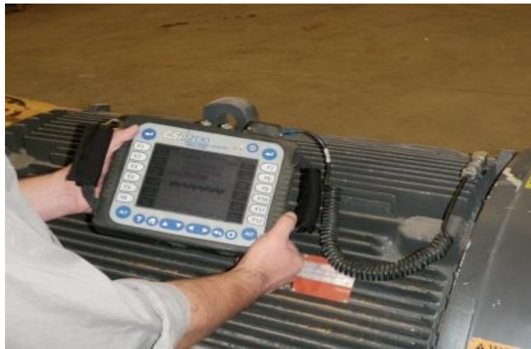
Figure 7 : Vibration analysis equipment
