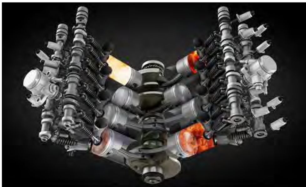
Figure 2.1 Bentley Continental V8 engine with variable displacement system
