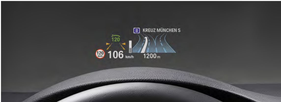
Figure 1.1: The head-up display of BMW.
