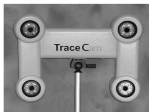
(b) Four-camera head AICON DPS (1300 × 1000 pixels).
