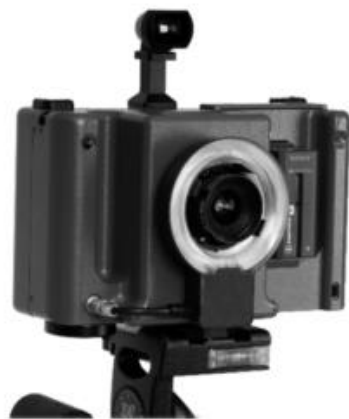
(a) Metric camera GSI INCA 3 (3500 × 2350 pixels).
