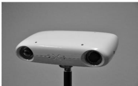
(a) Metric stereo camera AXIOS 3D CamBarB2 (1392 × 1040 pixels).
