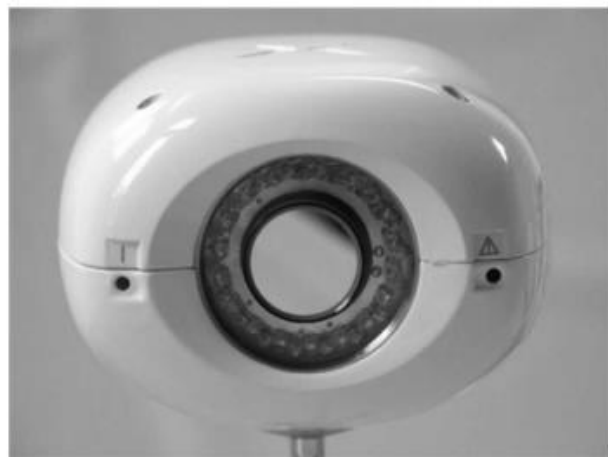
(b) Metric video camera AXIOS 3D SingleCam (776 × 582 pixels).
