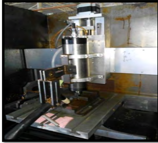
Figure 2.3.: Mini CNC Machine with plasma torch attached in front of the spindle
