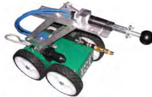
Figure 2.6: DuctCleaner Robot uses wheels to move around (LIFA AIR, 2008).
