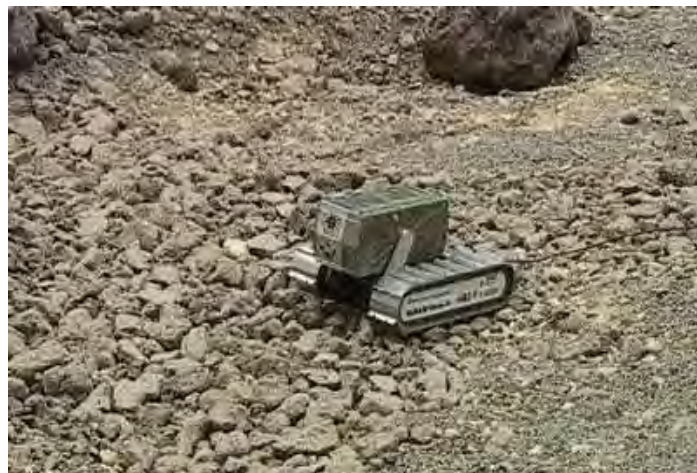
Figure 2.7: Nanokhod uses tracks to perform its locomotion (ESA, 2006).
