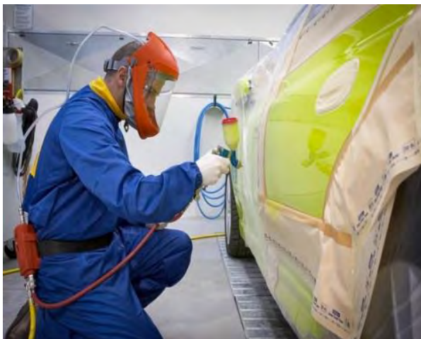
Figure 1. 2: The image of the spray painting process of the car at the garage ( http://www.pandorapigments.com )
