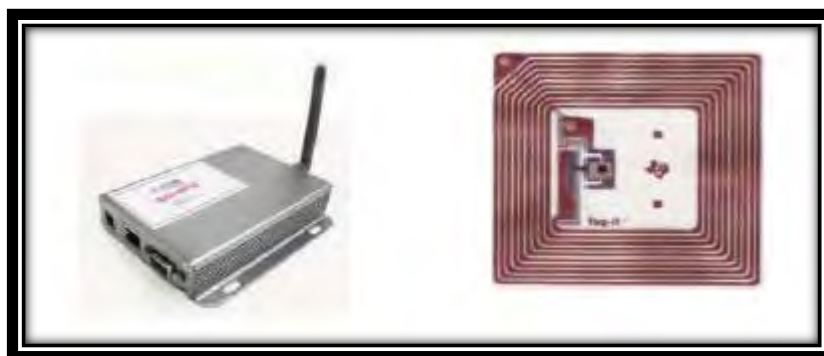
Figure 2.1: RFID Reader and RFID Tag
