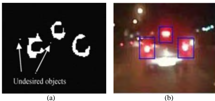
Figure 2.3: Example of detected brake lights. (a) The group of white pixels. (b) The detected brake lights are indicated by the bounding boxes [5]
