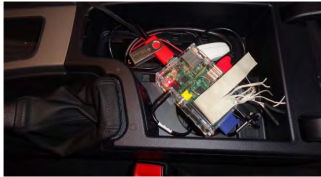
Figure 2.1.7: Mounted Raspberry PI in the armrest
