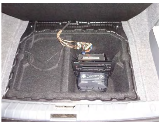
Figure 2.1.6: Trunk with relocated OEM Radio/CD player
