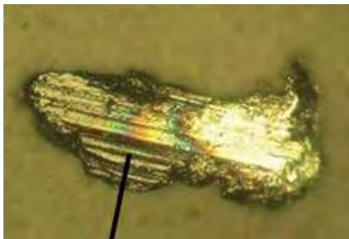
Figure 2.4: Severe sliding wear particles (Fitch, 2013)
