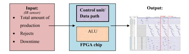
*Figure 1.1: Block diagram of control unit/data path for production monitoring system.*
