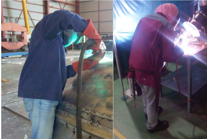
Figure 1.2: Welders perform the SMAW process in awkward postures.
