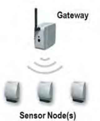
Figure 2.1 WSN Components, Gateway, and Distributed Nodes. [3]
