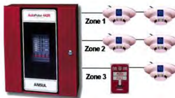
Figure 1.1 Conventional wired fire alarm system. [1]
