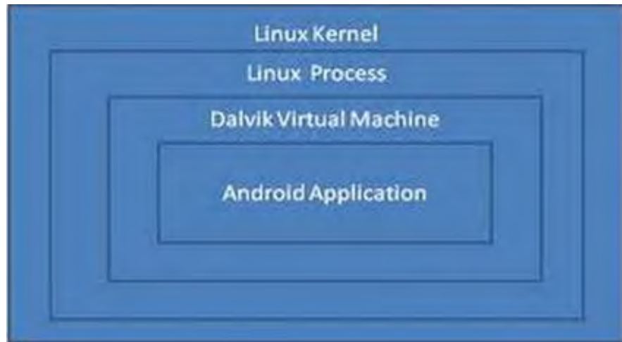
Figure 2.3: Dalvik virtual machine architecture [6].
