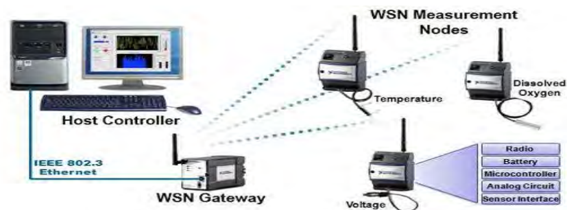
Figure 2.1: Basic Wireless Sensor Network (WSN) system
