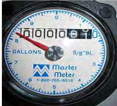
Figure 1.1: A typical water meter register showing a meter reading of 8.3 gallons. Notice the black "1" on the odometer has not yet fully turned over, so the red hand is read in its place.
