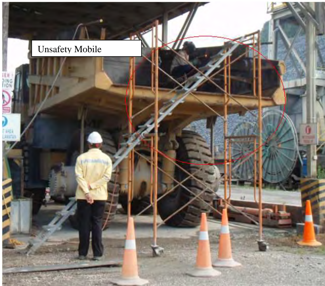
Figure 1.0: Existing Safety Mobile Platform
