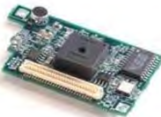
Figure 2.2: Acoustic wireless sensor device [13].
