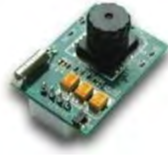
Figure 2.3: Camera-based wireless sensor device [13].
