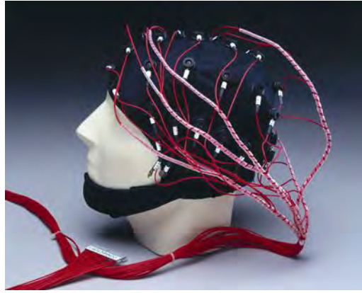
Figure 2.4: Sample EEG cap technology [2]
