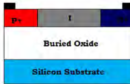
Figure 2.4: Optical modulator of PIN structure
