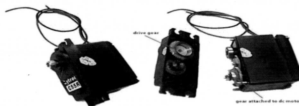
Figure 2.1: The standard DC motor with gearing
