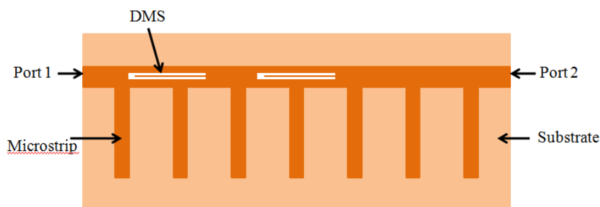
Figure 2.4: DMS structure on the microstrip.
