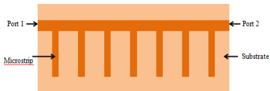
Figure 2.2: Example of planar microstrip band pass filter.
