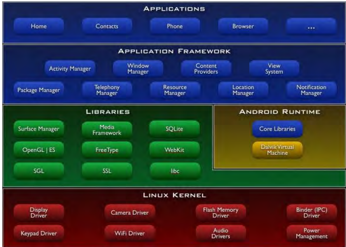
Figure 2.1: Architecture of Android System [1]
