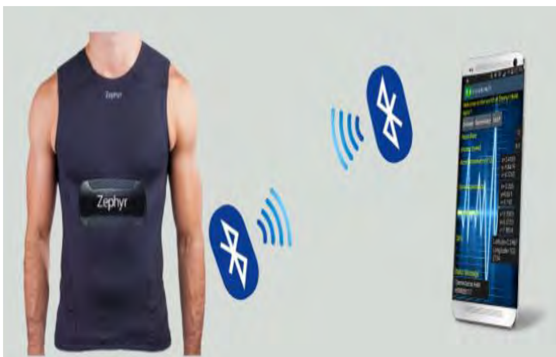
Figure 4.1: Hardware using Bluetooth communication with smartphone device.
