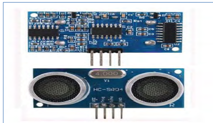
Figure 2.6: Product Layout of HC-SR04
