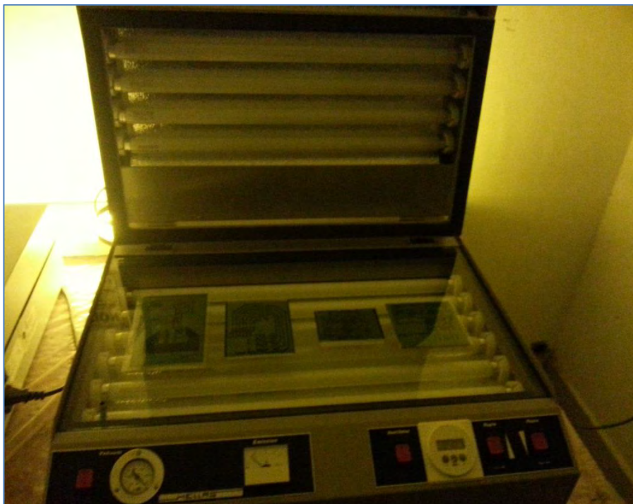
Figure 3.10: PCB board in the UV machine
