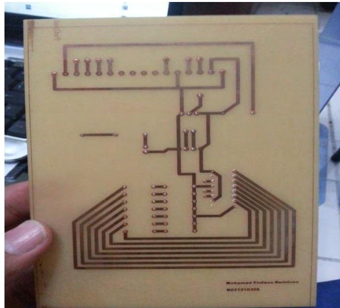
Figure 4.10: Complete Drilled Board
