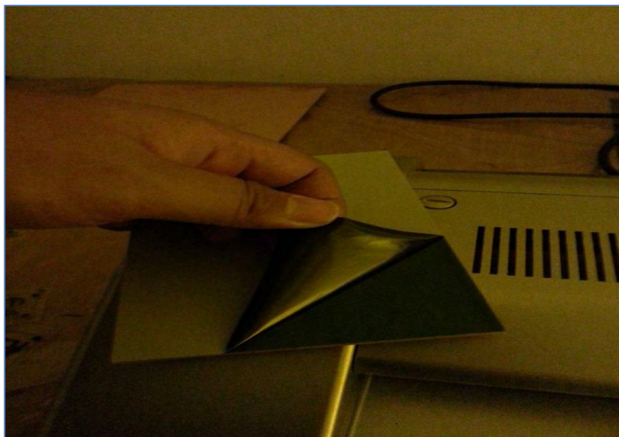
Figure 3.9: Protection layer remove in dark room
