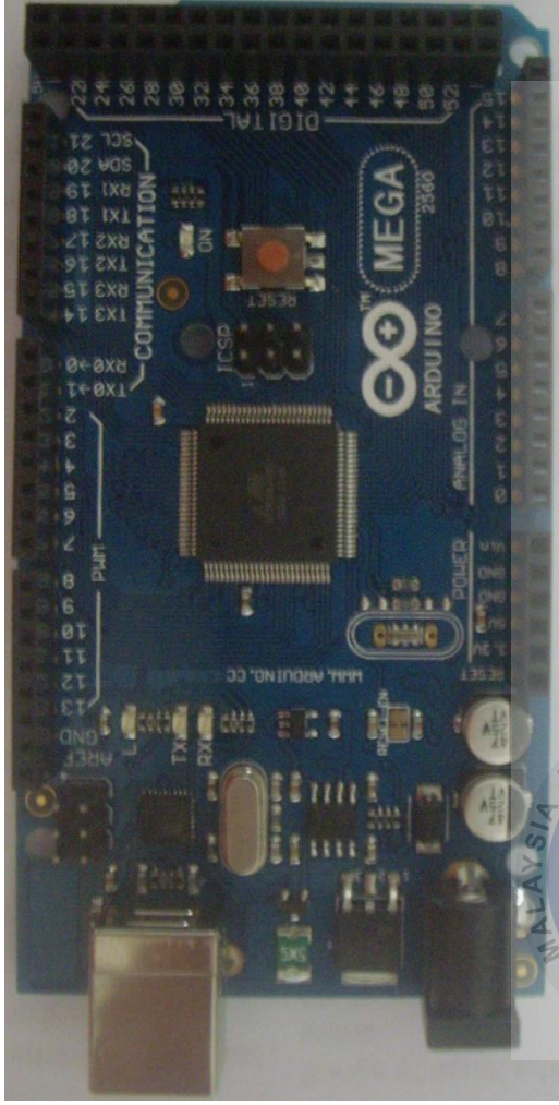
Appendix C Top layout of Arduino Mega 2560
