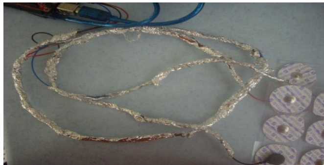
Figure 4.14: Wire shielded with aluminium foil
