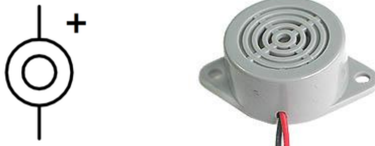
Figure 2.7: Buzzer or beeper
