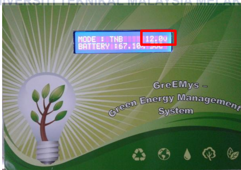
Figure 4.3: Display properties of voltage from battery.
