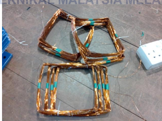
Figure 3.17: Phase group of winding for five-phase motor
