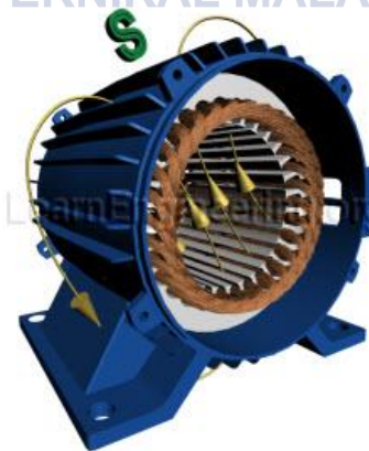
Figure 2.5: Rotating magnetic field produce in an induction motor [2]
