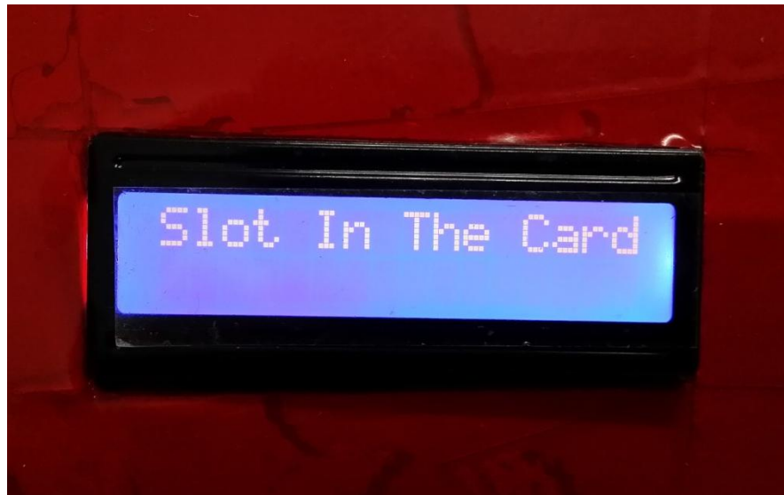
Figure 4.9: LCD Display When There Are No Card Inserted
