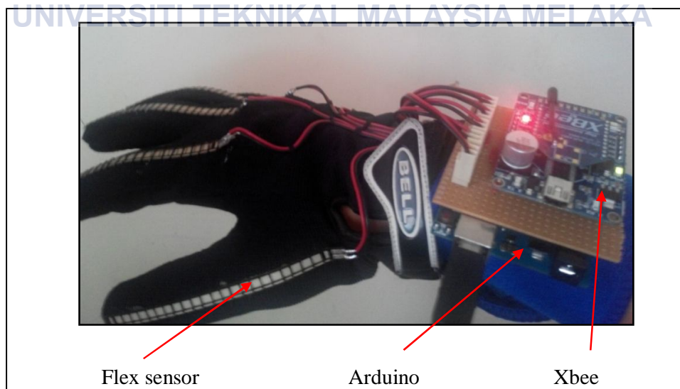
Figure 3.8: Master data glove
