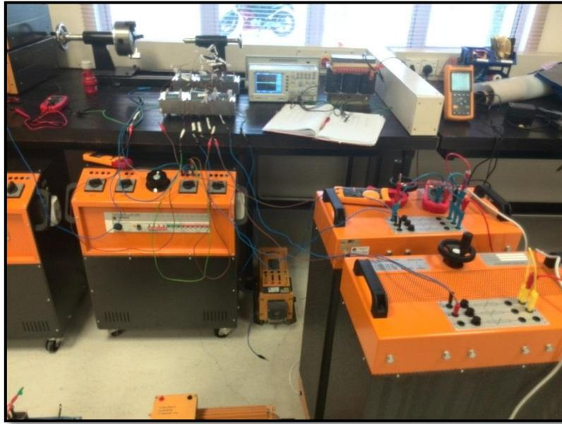
Figure 3.15: Hardware setup for resistive load testing
