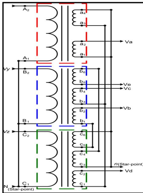
Figure 3.2(a): Transformer winding arrangement in wye-wye connection [1]
