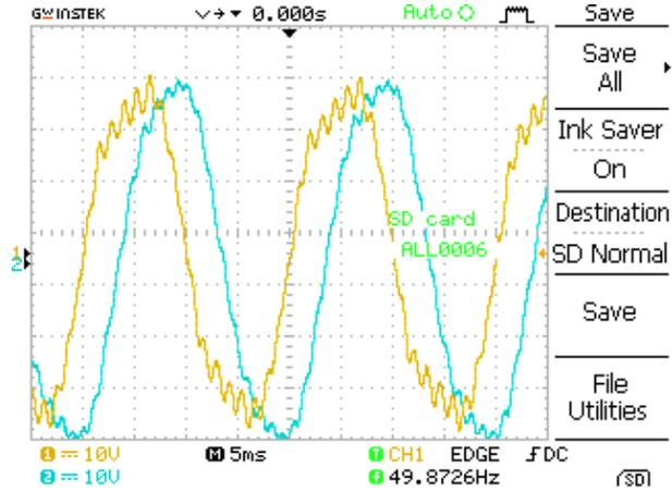
Figure 8: Output waveform for two phases of five phase transformer connected to four unfilled slots five phase induction motor
