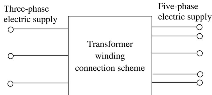
Figure 2.11: Block representation of the proposed system [1]
