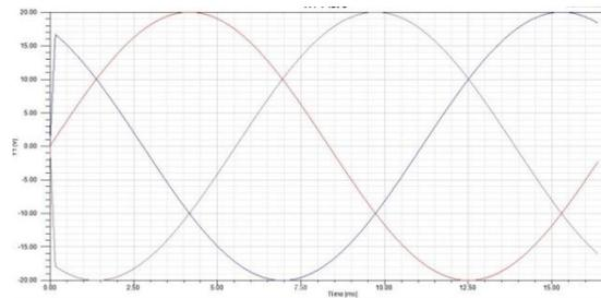
a) Three phase input for five phase transformer
