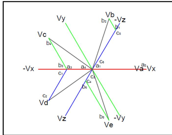
Figure 3.3: Phasor diagram of the transformer connection in wye-wye connection [1]
