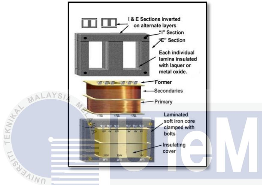
Figure 2.3: The construction of the transformer [8]
