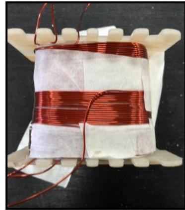
Figure 4.10: Copper wires was not arrange fitted
