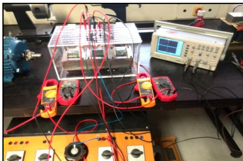
Figure 3.13: Hardware setup for no load testing
