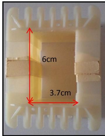
Figure 3.6: Transformer bobbin
