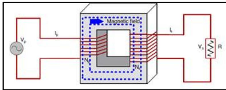
Figure 2.2: Transformer schematic [8]
