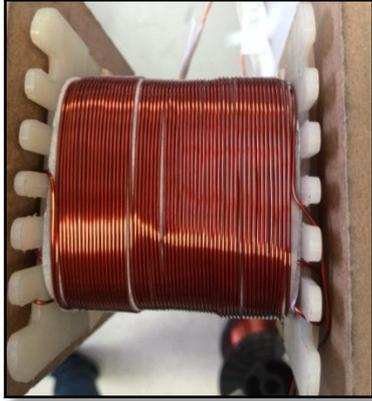
Figure 4.9: Copper wires was not arrange neatly
