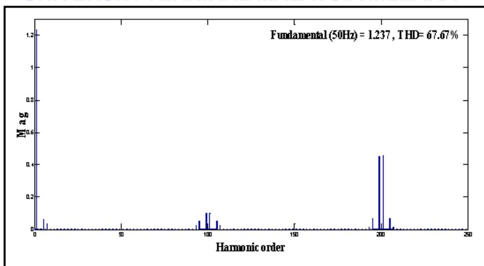
Figure 4.15: THD for phase current (inverter) [23]
