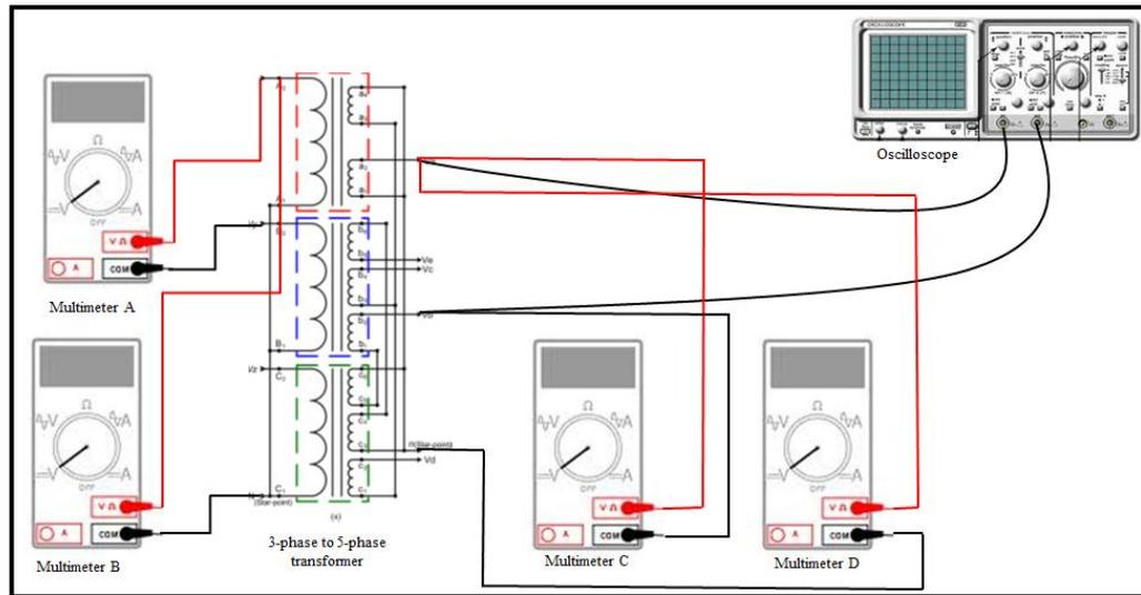
Figure 3.12: Circuit connection for no load test
