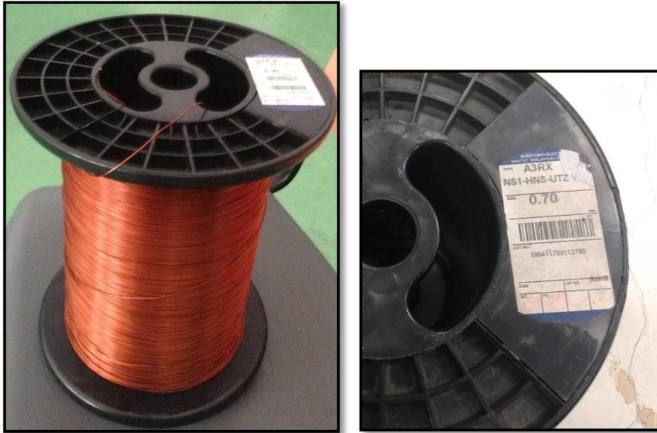
Figure 3.7: 0.7mm enamelled copper wire
