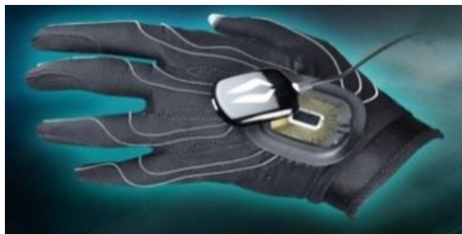
Figure 2.1: Back glove as controller
