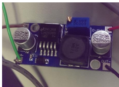
Figure 3.17 – Step-down voltage regulator
