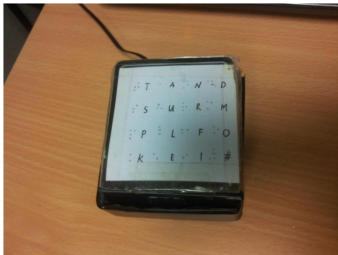
Figure 3.24: Modified Keypad with Braille Code
