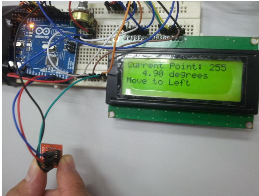
Figure 4.2: Compass Reading When Point to North
