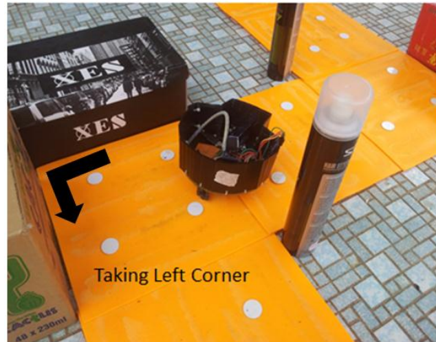
Figure 4.13: Mobile robot takes left corner
