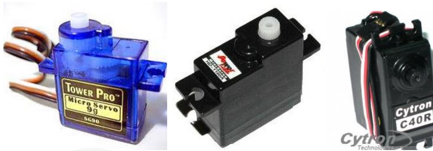
Figure 3.15: SG90 micro servo, HD 1160A micro servo and C40R RC hobby servo
