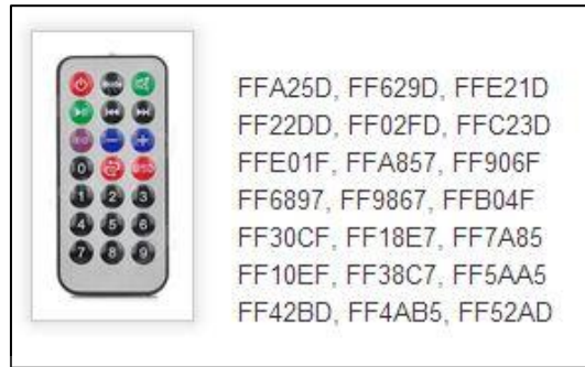
Figure 3.13: IR remote keypad with serial code for each button
