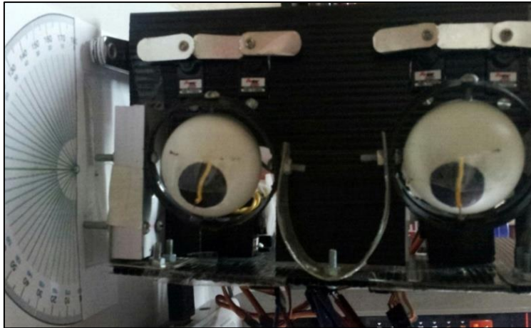
Figure 3.27: Front view of eyeball for down position
