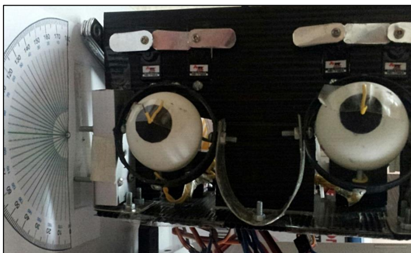
Figure 3.26: Front view of eyeball for up motion
