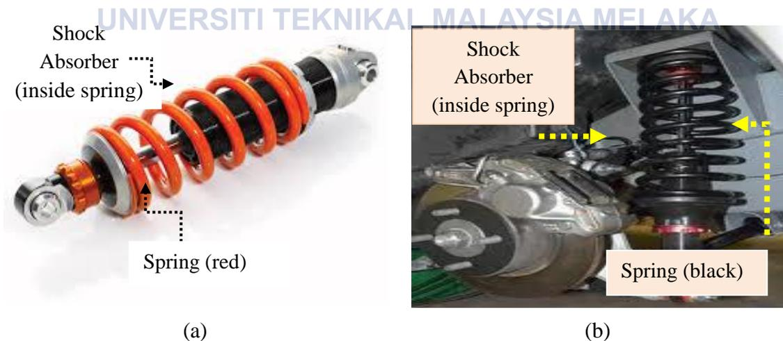
Figure 1.2: (a) Diagram of spring and shock absorber [20], and (b) How absorber and spring are attached to a vehicle [21]
