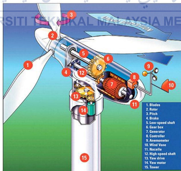
Figure 2.8: Parts inside the wind turbine
