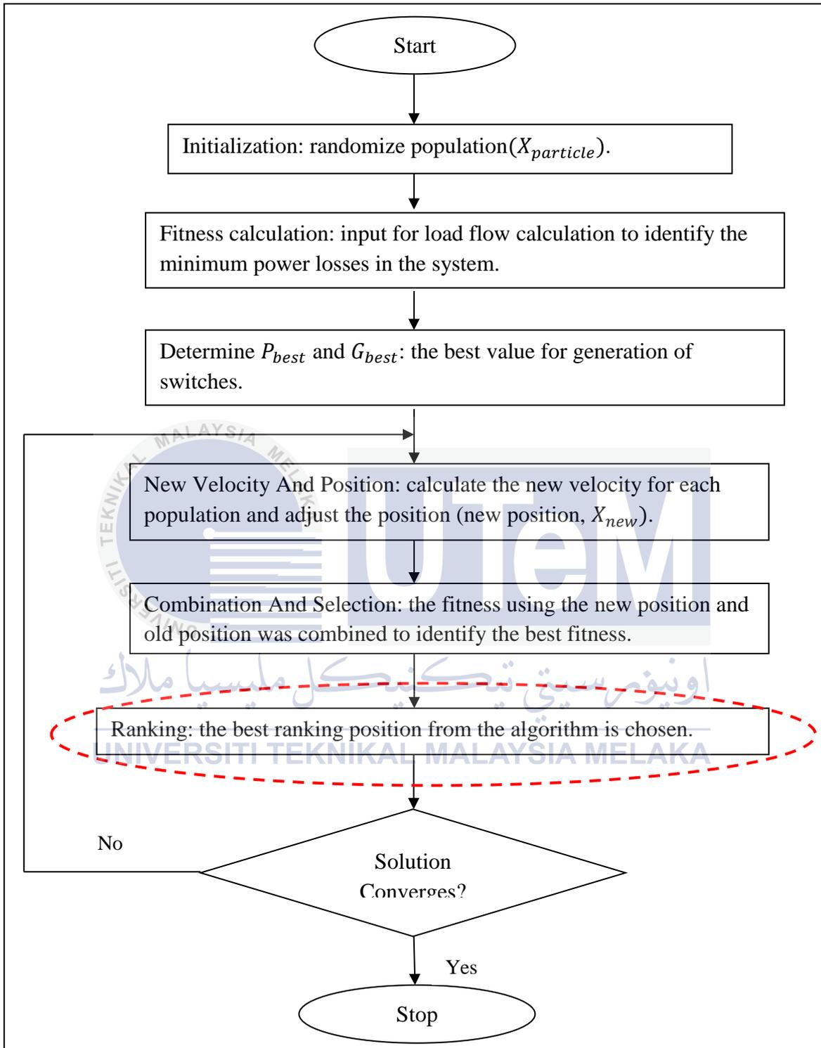
Figure 3.2: Implementation of REPSO in Network Reconfiguration.
