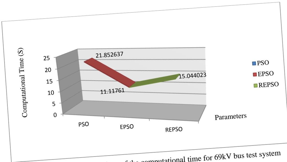
Figure 4.8 : The comparison of the computational time for 69kV bus test system
