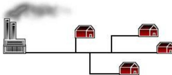
Figure 2.1. Radial configuration
