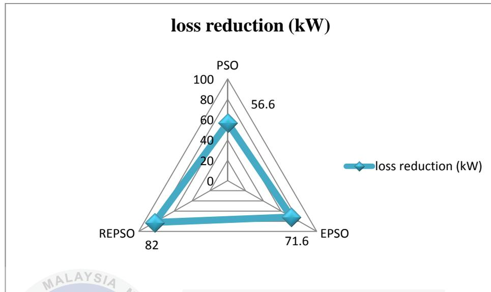
Figure 4.4: The comparison of total power losses reduction between PSO, EPSO and REPSO algorithm.
