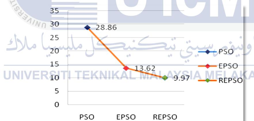
Figure 4.5: The comparison of the convergence time between PSO, EPSO and REPSO algorithm
