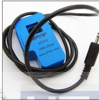
Figure 3.9: SCT013, 100A:50mA current sensor [29]
