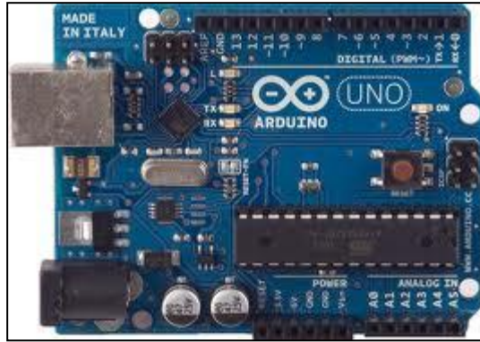
Figure 3.8: Arduino Uno with variety of input and output pins.
