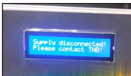
Figure 4.11: System warns the consumer that supply is already disconnected.
