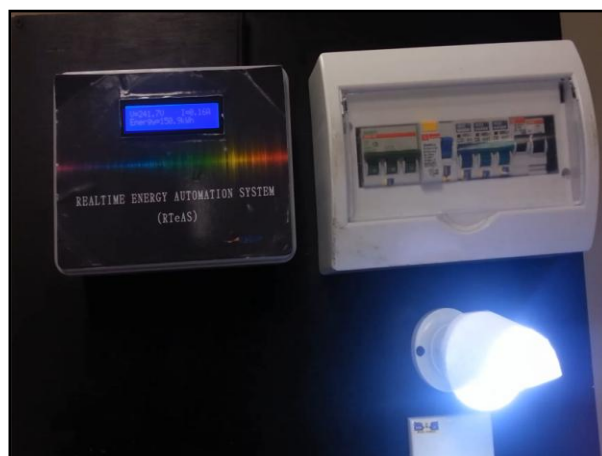
Figure 4.2: Smart Meter System with 100W light bulb.
