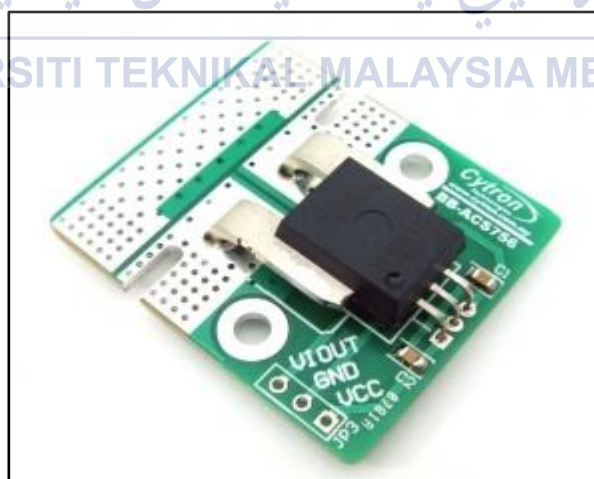
Figure 3.7: Hall-effect linear current sensor.
