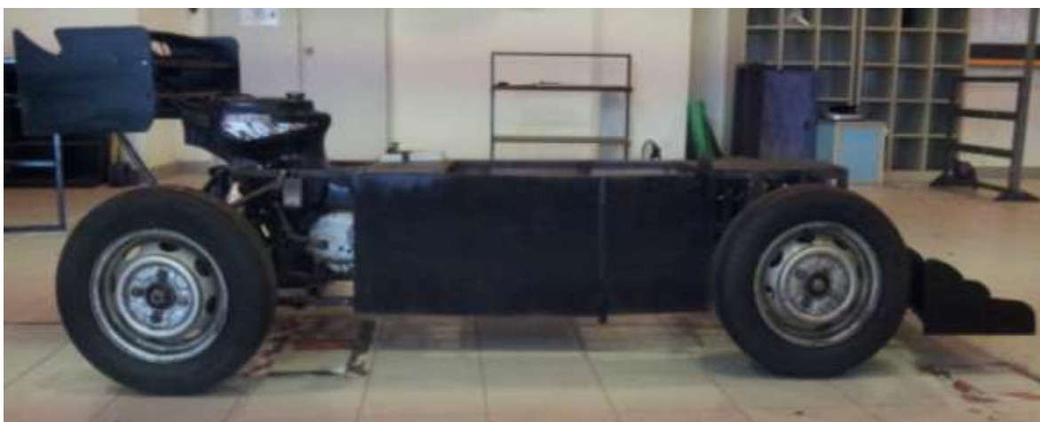
Figure 4.9 (a): Side View Of Fabricated Chassis
