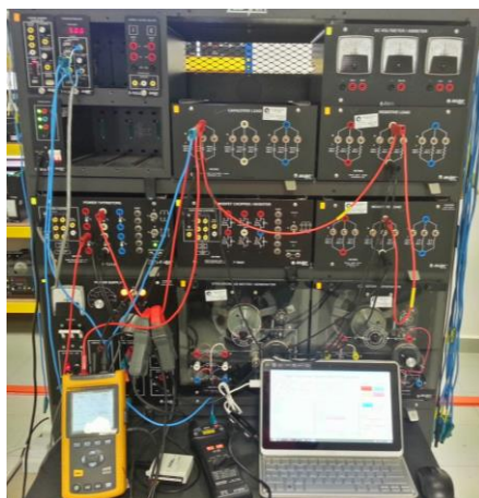
Figure 3.15: Experimental Set Up for Full Wave Controlled Rectifier
