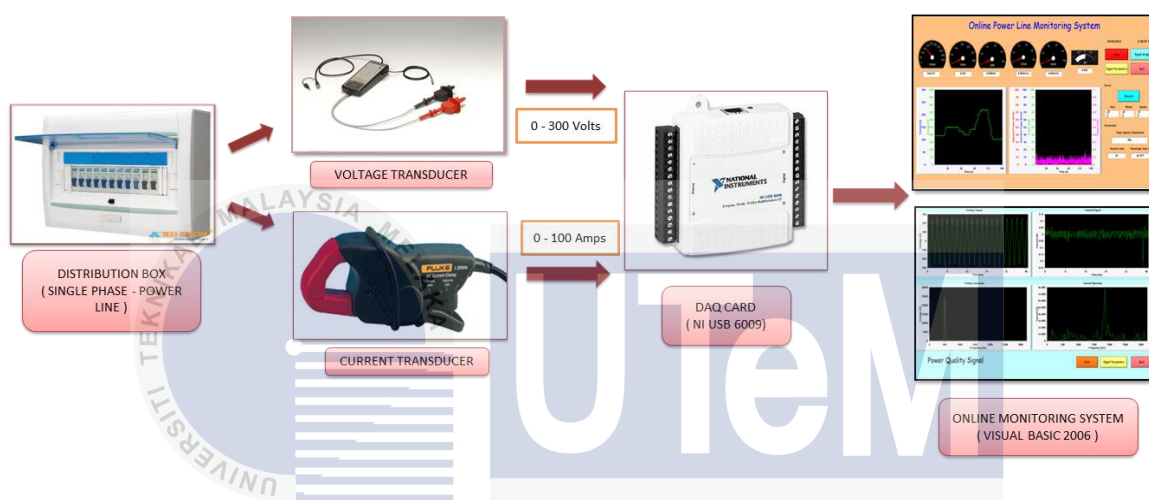
Figure 3.1: Block Diagram of Real Time Power Quality Monitoring System
