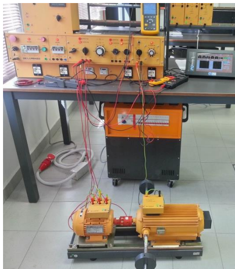
Figure 3.8: Experimental Set Up for Blocked Rotor Test
