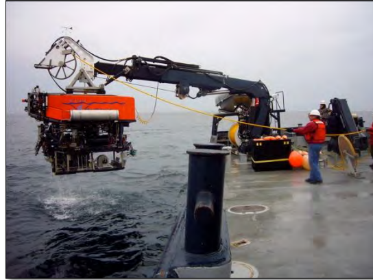
Figure 2.2 The Stem Mounted Crane
