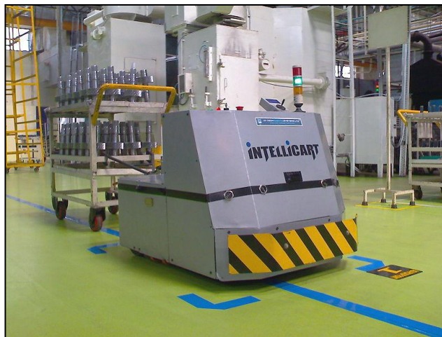
Figure 1.1: An example of mobile robot or Automated Guided Vehicle (AGV) ( www.wheelomania.com , 2013).
